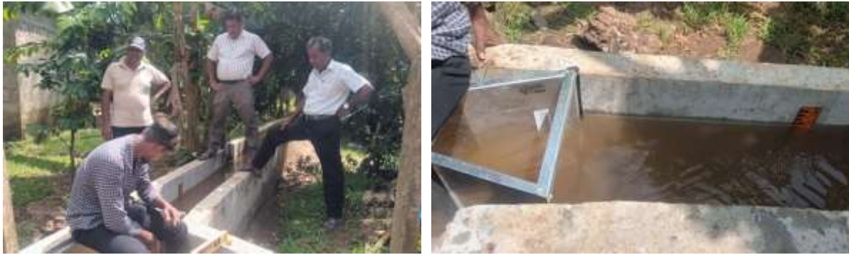
Plate 17: Calibrate Canal Gauge - Karangahawewa, Trinco- EP
